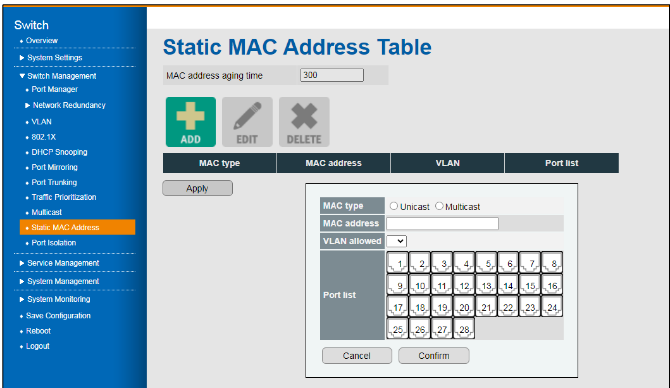
Figure 30 Switch Management > Static MAC Address Menu
