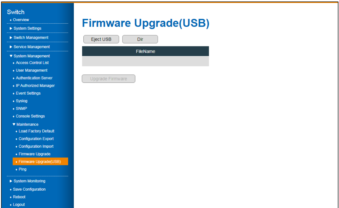
Figure 51 System Management > Maintenance > Firmware Upgrade (USB) Menu
